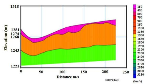
Fig. 5 Tomographic section of subsurface lithology
